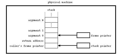
Machine registers are reserved for the accumulator, stack pointer and frame pointer.
