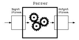
Any stream can be used as input for a parser. A single object stream can be the output stream for one parser and the input stream for another. This creates pipelines of stages transformations, each stage being driven by a particular parser. The input end of a pipeline can be fed from a file input stream (converting the contents into a stream of integers) and the output end can be connected to file output stream (converting a sequence of objects back into a textual or binary form).
